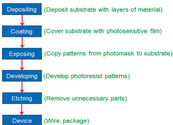
Figure 1. A typical MEMS fabricating process
