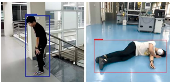
Figure 9. Results of our fall detection based on YOLOv4-tiny; the left image is a people detection in a blue box, and the right image is a fall detection in a red box.
