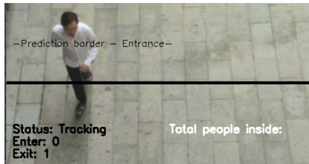
Figure 3. Experimental result of the system using proposed methods (SSD and Centroid Tracker) at Eastern International University
