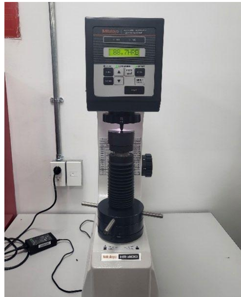
Figure 2. Measuring the workpiece hardness
