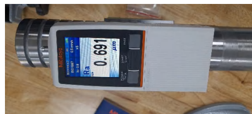
Figure 9. Measuring surface roughness
