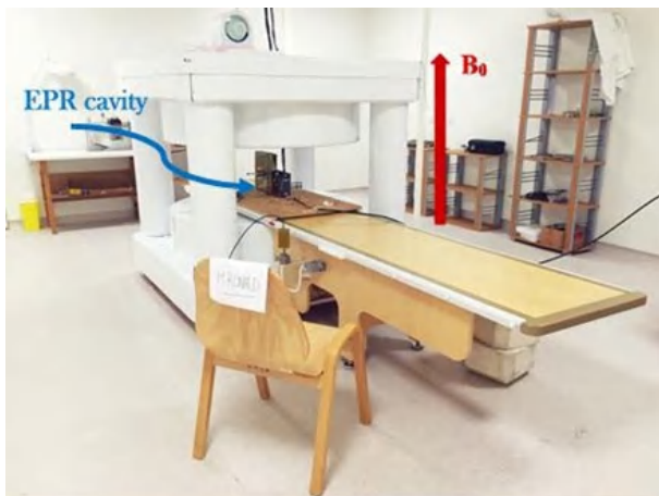
Figure 2. Illustration of the MRI 0.2T system, with the microwave cavity
