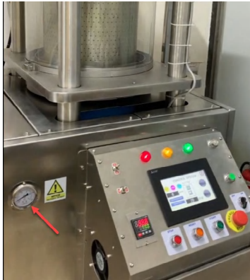
Figure 15. The analog pressure gauges
