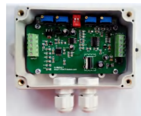
Figure 5. LoadCell Weight Transmitter Amplifier JY-S60
