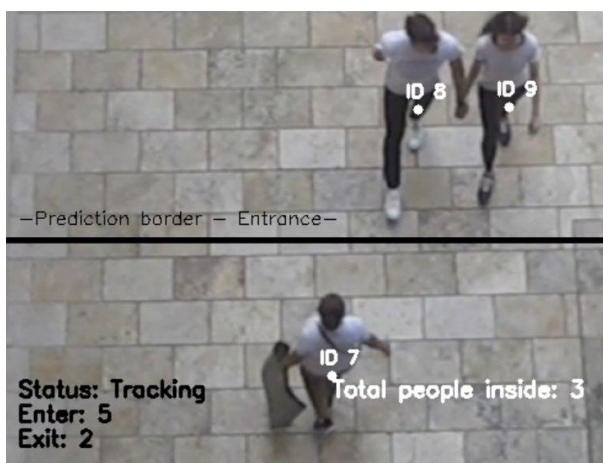
Figure 2. Testing result of the system using proposed methods (SSD and Centroid Tracker) from a video
